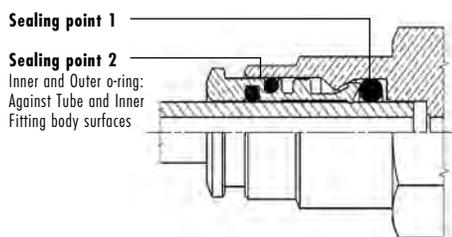
Possible micro scratches on the tube are eliminated due to 2 o-rings at Sealing Point 2
