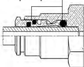
**Sealing point 1** is the traditional sealing point on a push-in fitting. While the additional **Sealing point 2** works on fresh tubing (non scratched), as well as keeping dirt and debris from entering tube gland and fitting
