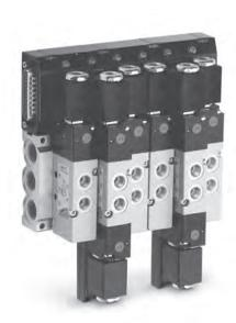
This Plug-In system, realized with electropneumatically operated valves Series 3, G1/8 port, is delivered completely assembled and tested. It allows the mounting of up to 22 valve positions (with two SUB-D 25 RIGHT and LEFT connectors). The electrical part is based on printed circuit boards.
