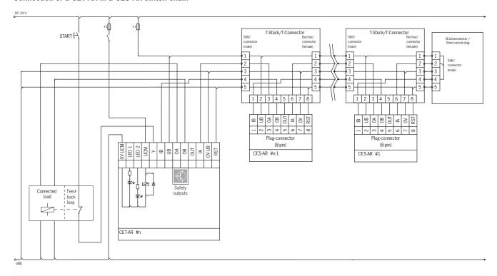
**Important**: The subsystem CET-AR complies with PL e according to EN 13849-1. To integrate the subsystem in a category 3 or 4 structure, it is necessary to monitor the downstream load (the feedback loop must be monitored).
