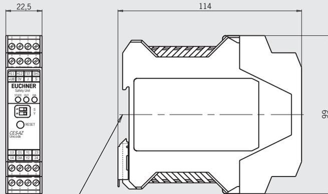
Suitable for 35 mm DIN rail according to DIN EN 50022-35
