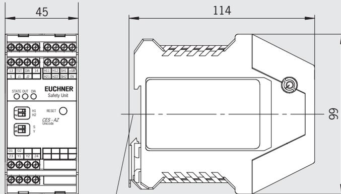
Suitable for 35 mm DIN rail according to DIN EN 50022-35
