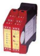
When emergency stop is activated, 2 NO contacts immediately open, 2 additional contacts open after a preset time delay. This redundant time delay can be set from 0.005 to 600 S, in 64 steps. Both timers must be set the same.
